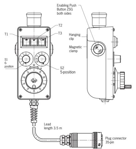
2 Selector Switches, 6-position (X, Y, Z, 4, 5, 6) and 5-position (0, 1, 10, 100, 1000)
